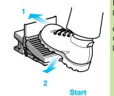
Positive action is required on the toe plate 1 before the pedal 2 can be depressed to start the machine.
